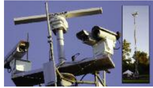
ACCIPITER RADAR INTEGRATED WITH OTHER SENSORS
